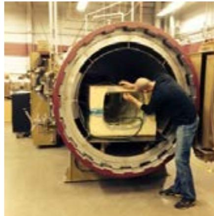
Students at the University of Utah used LAST-A-FOAM® to build a mold for the carbon fiber outer shell of their formula SAE racecar.
