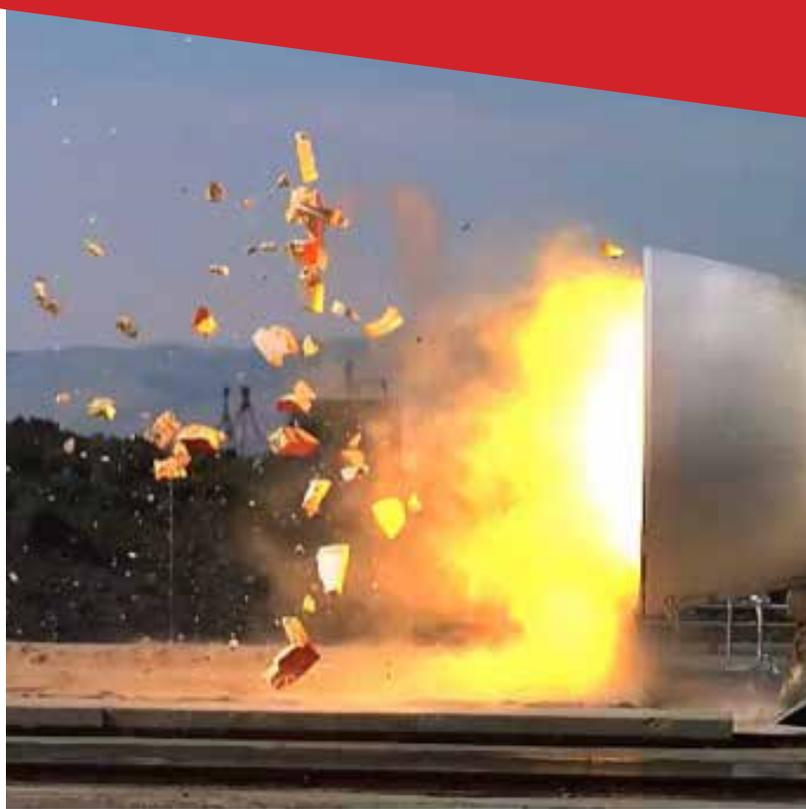
*L: QM-2 Static Test - High speed video of nozzle plug blow out. R: Nozzle blow out demonstration. Photos provided by Orbital ATK*
