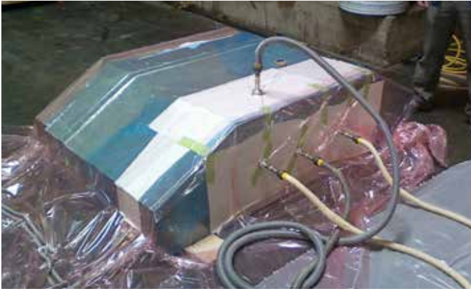
LAST-A-FOAM® Tool in Bagging Layup Process
