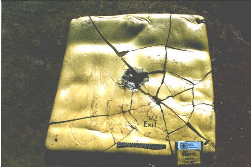
FIGURE 5 UPPER SIDE OF RPF BLOCK FRACTURED BY DETONATION OF 30 GRAMS OF PETN POSITIONED 12 INCHES BELOW THE CENTER OF THE PATTERN.
